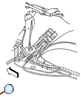
5. Align the module to the vehicle antenna module bracket.
